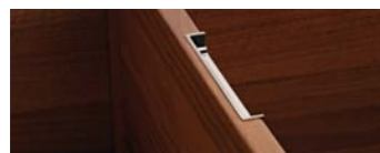
Edge Inset Handle. 233 (96mm Centre/135mm overall) S/Steel effect handle can be used on door thickness 18mm or greater, in conjunction with aluminium top and side spacer trims (30mm planning space)
